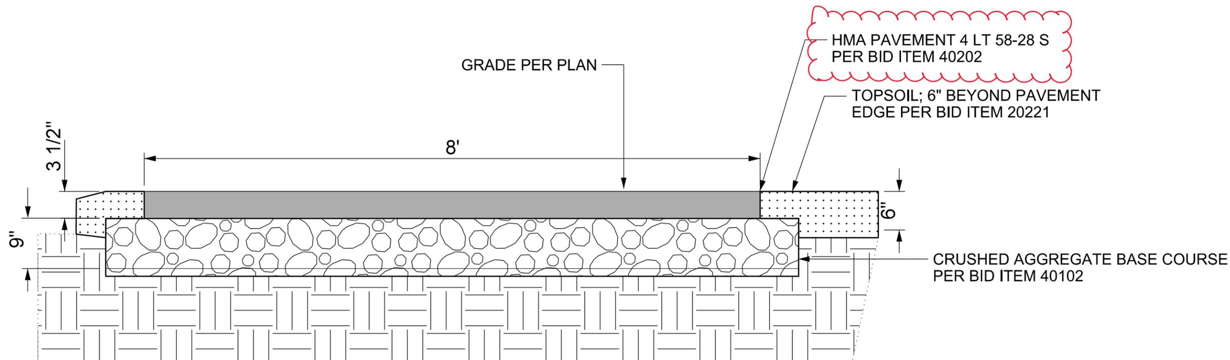
① **TYPICAL ASPHALT PATH SECTION**
